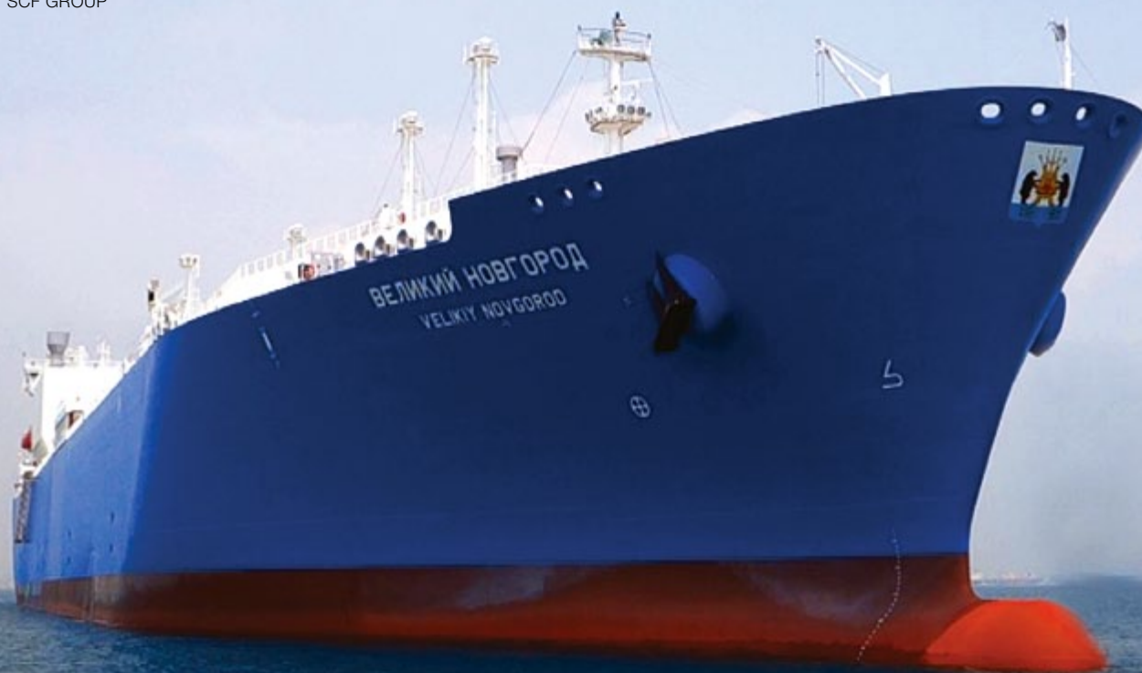
Velikiy Novgorod , an Atlanticmax Ice2-class LNG carrier designed for the year-round transportation of gas. The vessel is chartered to Gazprom under a long-term contract
